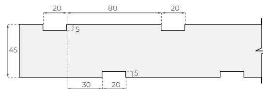
Double Bevel Double Castellated 45x45 H3.2 Treated FJ Pine
