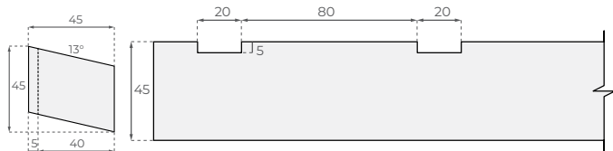
Double Bevel Single Castellated 45x45 H3.2 Treated FJ Pine
